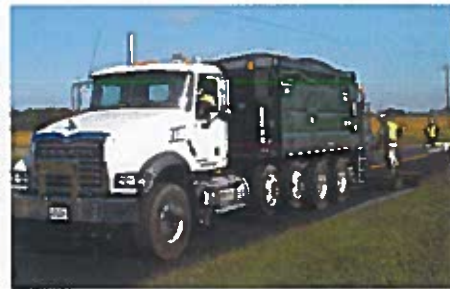
Typical truck used in slurry seal operations.
